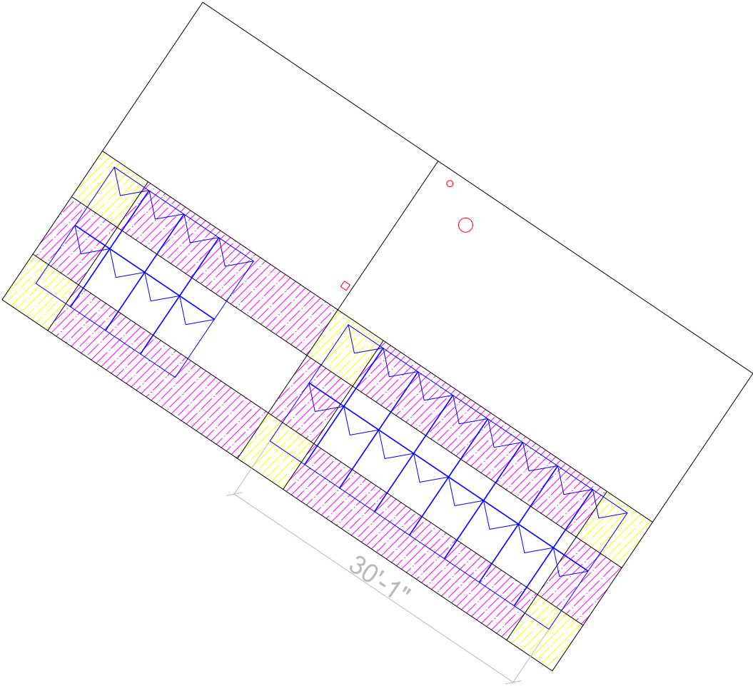
3 PV-2 PV SITE PLAN WITH MODULE LAYOUT & ATTACHMENT ZONES
